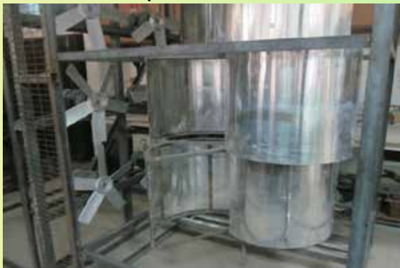
Vertical Axis Wind Turbine
